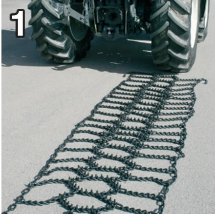
1 Put the chains behind the tire with the fasteners against the tractor and the studs facing up.
