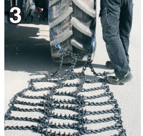
3 Put the rope on the top of the tire.
