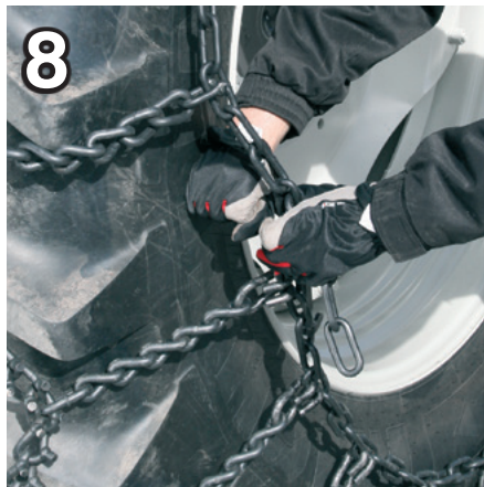
8 A good rule is that your hand should fit between the tire and the chain. Do not tension too tight. Hammer the plugs of the couplers.
