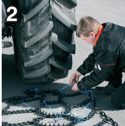
2 Fasten the rope in the middle of the chain.
