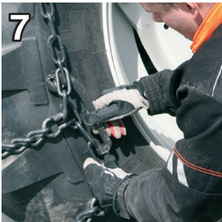
7 Fasten the chain with the fasteners, inside first and then outside.
