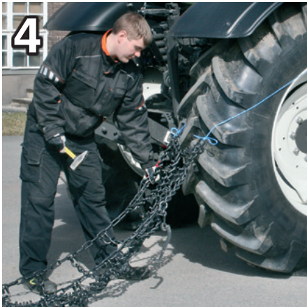
4 Drive forward one circuit, keep the chain narrow.
