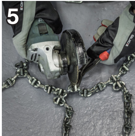
5 In most cases the chain must be cut to fit perfectly. Always make the cut from a studded link. Don't cut the chain too short.
